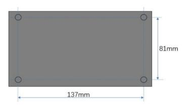
步骤 2. 使用钻孔设备在面板上已标记的安装孔位置钻孔。Use drilling equipment to drill holes in marked mounting positions on the panel.
